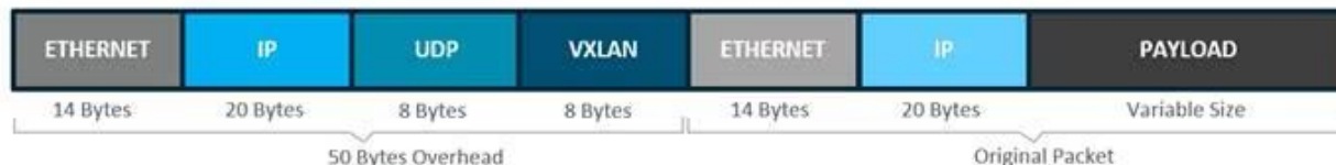
Figure 6. Fabric VXLAN (VNI) Encapsulation Overhead
