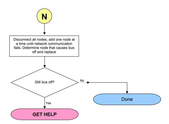
**Start 2:** DeviceNet Plant Floor Troubleshooting Flowchart (Intermittent Failures)
