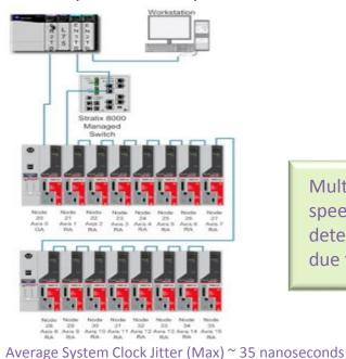
Multiply your application speed by this value to determine position error due to network jitter
