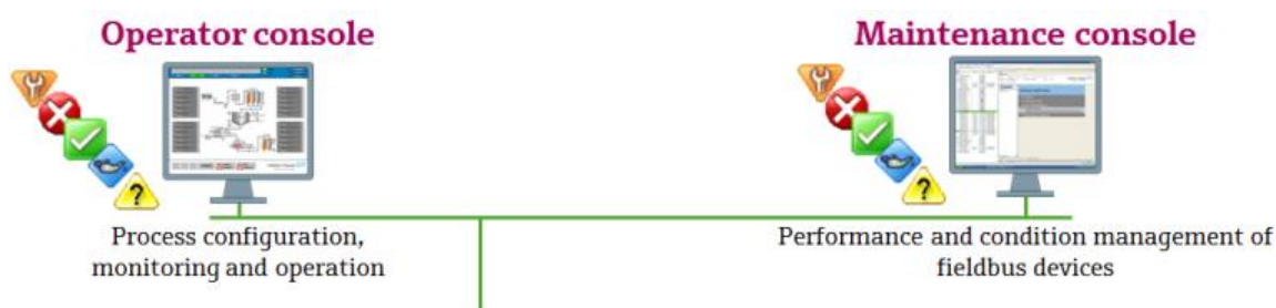
Figure 3: Operator and maintenance console, both showing diagnostic information
