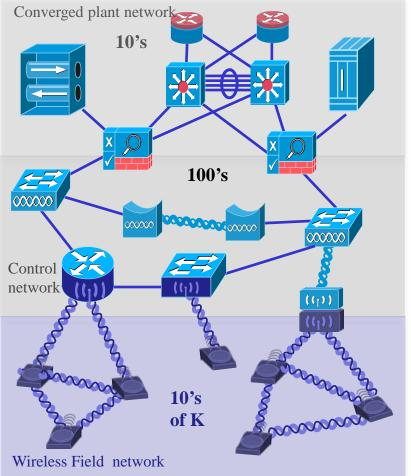
**Converged Plant Network** High availability Flow Isolation **Guaranteed Bandwidth** IP based Control Network Autonomic, zero touch commissioning Time Sensitive Networking for critical apps Packet Reliability IPv6-based Wireless Field Network Deterministic, Autonomic, Secure Large Scale for Monitoring (RPL) Backward Equivalence (TSCH)
