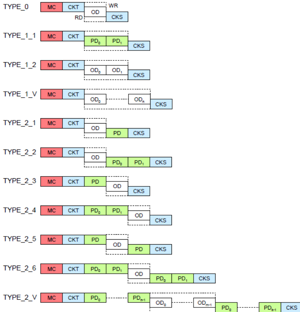
Figure 9: IO-Link transmission frames
