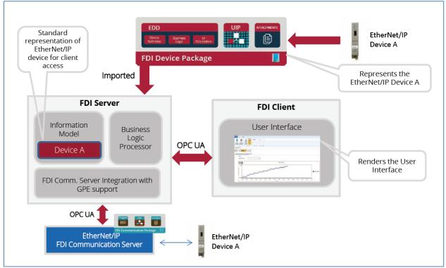
**FDI Device Packages** for EtherNet/IP device are imported into the FDI Host system. The Device Definition and Business Logic are used exclusively by an FDI Server and the User Interface Description (UID) is processed by the FDI Server and transferred to the FDI Client. Each EtherNet/IP Device package instance is represented in the FDI Server Information model and provide an access to the FDI Client.
