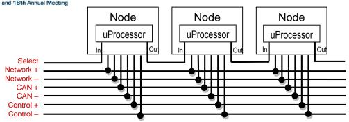
Select Line Messages are received on the Select In line. The device services the message, and after processing is complete, the message is retransmitted on the Select Out line. The result is sequential message delivery from "left to right".
