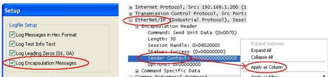
Figure 3 – Configure Wireshark for use during EtherNet/IP Conformance Testing
