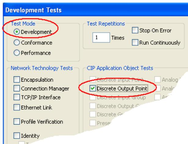
Figure 2 – Use Development Mode for Flexible, Focused Testing of CIP Functionality
