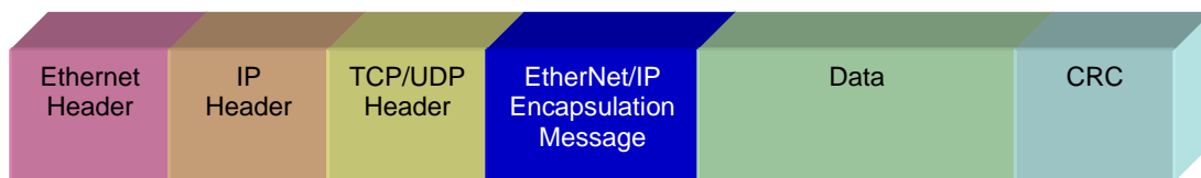
Figure 10 - Layering in an EtherNet/IP Message
