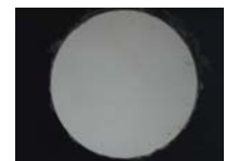
Figure 7 Fiber polished 0.3 micron paper
